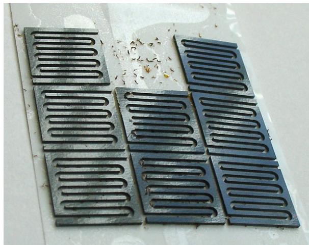
Fig. 3. Machined Cirlex ® fluidic walls. Each design is 1 cm \times 1 cm in dimension.
