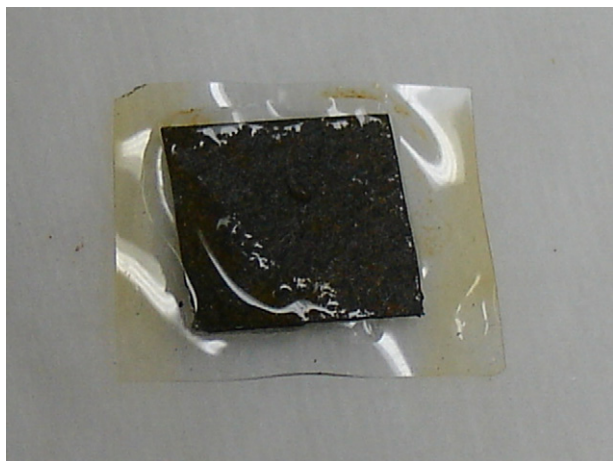
Fig. 8. The finished MEA. The liquid shown on the MEA is water.
